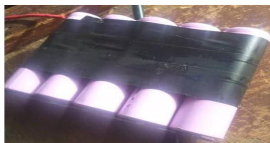
Figure 5: Li-ion batteries connected in parallel.
