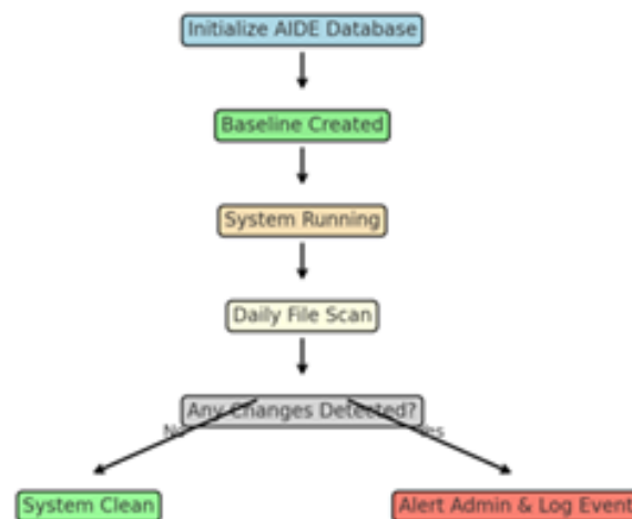
Figure 1: AIDE compares system files with a baseline database to detect unauthorized changes.
