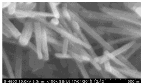
Figure 3: SEM image of iron oxide nanoparticles before calcinations
