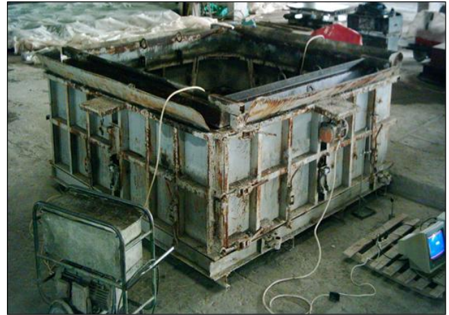
Figure 4: The view of the mold of precast concrete unit (box element)
