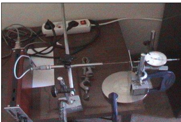
Figure 3: The set-up of calibration of the displacement transducer
