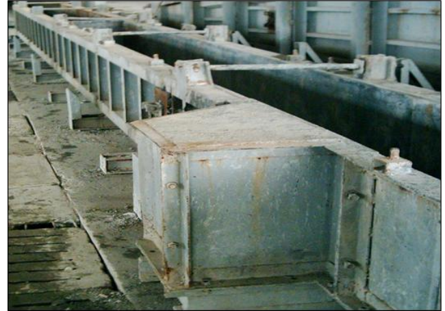
Figure 4: The view of the mold of precast concrete unit (column element).
