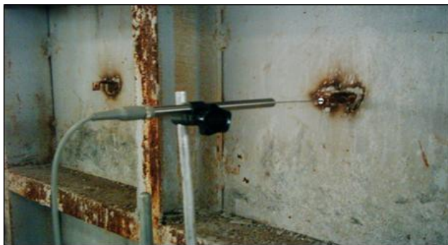
Figure 2: LVDT (Linear Variable Differential Transformer, Displacement Transducer)
