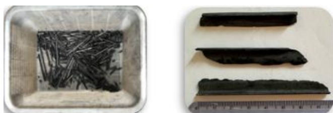
Figure 1: Buildup on the inner wall of the cracking furnace tube
