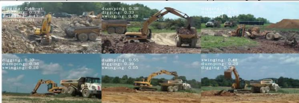
Figure 24: Long video demos of action recognition results on various scenes from the construction dataset: top predictions highlighted (Zhang & Zhang, 2021, p.55)
