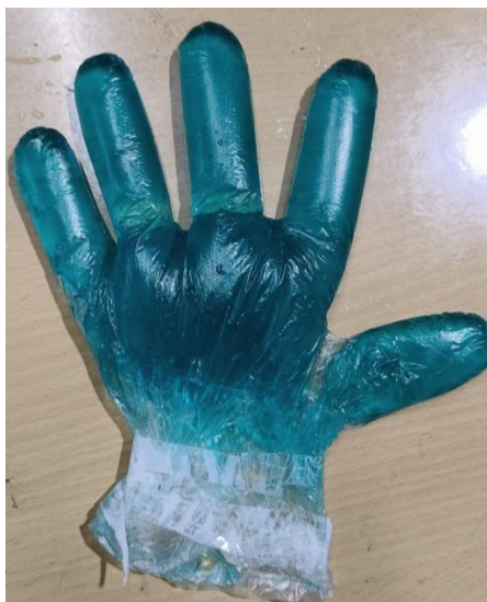
Figure 4: PCM gel encapsulated within flexible bags, moulded into the glove shape
