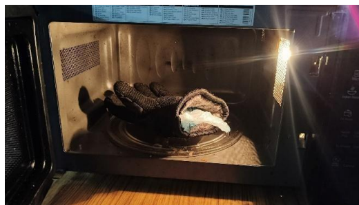
Figure 3: Convection-oven based heat-exposure testing setup used to evaluate the glove samples.
