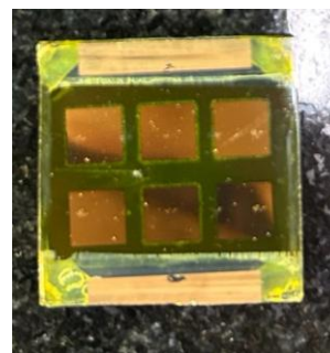
Figure 5: Encapsulated six-pixel perovskite module used for the LED demonstration.
