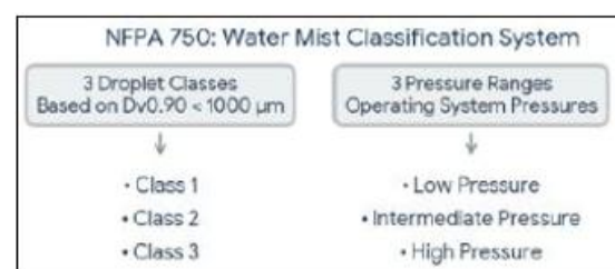
NFPA 750: Water Mist Classification System
