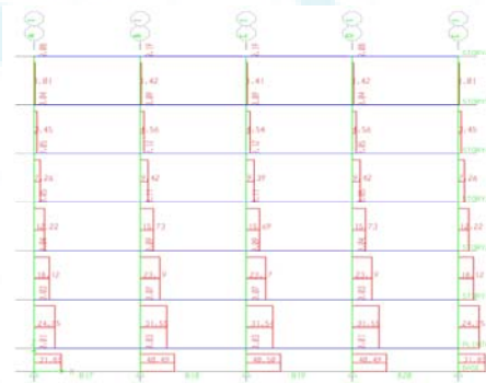
Figure 4.6: Distribution of axial force in column due to response spectrum earthquake load for 50 percent infill condition
