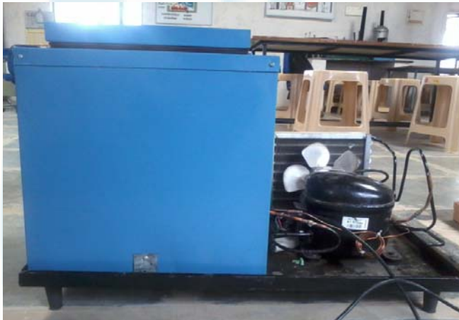
Figure 4: Photograph of Fabricated cold storage plant in Thermal lab
