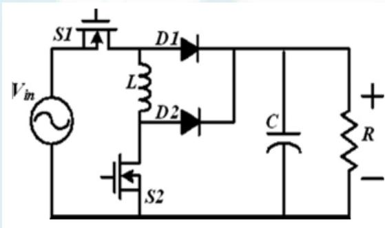
Figure 3: Bridgeless boost rectifier for energy harvesting
