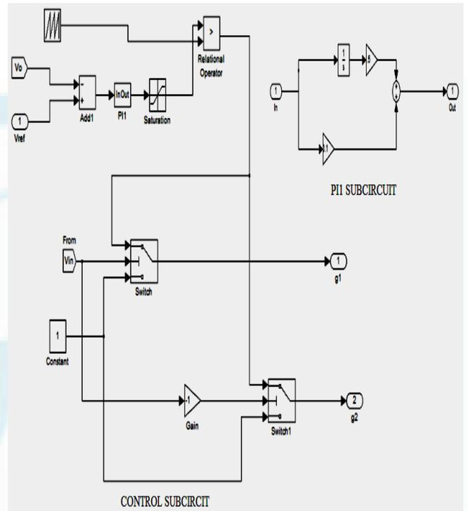
Figure 8: Simulation model of gate signal generation
