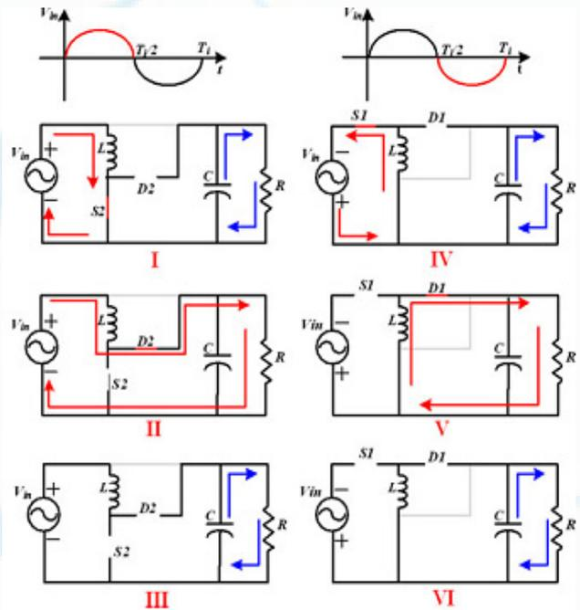
Figure 4: Operating modes of the proposed boost rectifier
