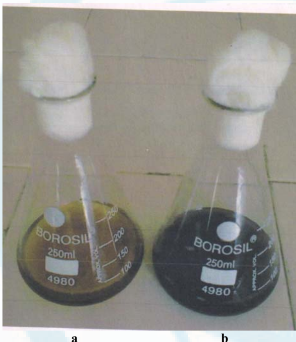
Figure 2: Silver Nanoparticles synthesis from leaf extracts a. Neem b. Papaya
