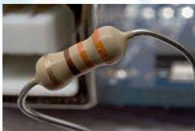
Figure 12: A typical axial-lead resistor
