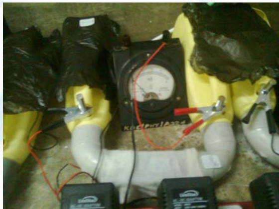
Plate 2.1: A Modified Electrochemical Cell for electrical resistivity (courtesy of Mutitu D. Karanja)
