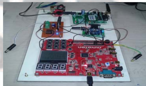
Figure 8: Picture of Base Station Module
