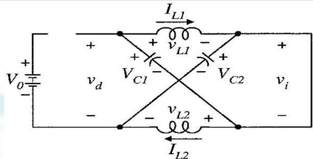
Figure 7: Equivalent circuit of the Z-source inverter viewed from the dc link when the inverter bridge is in the shoot-through zero state
