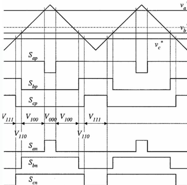
**Figure 9:** Traditional carrier-based PWM control without shoot-through zero states, where the traditional zero states (vectors)  $V_{111}$  and  $V_{000}$  are generated every switching cycle and determined by the references
