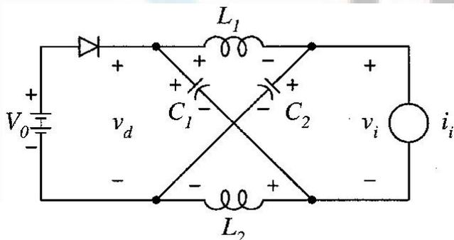
Figure 6: Equivalent circuit of the Z-source inverter viewed from the dc link
