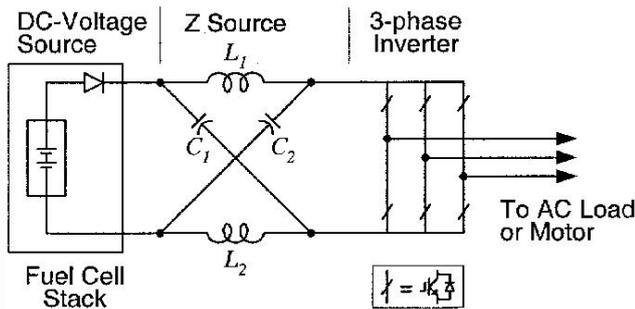
Figure 5: Z-source inverter for fuel-cell applications.
