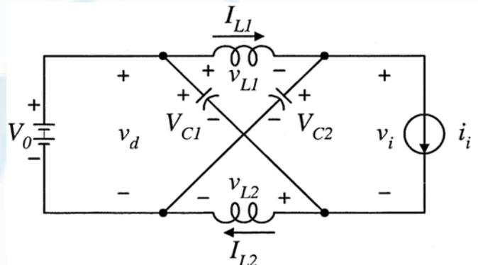
Figure 8: Equivalent circuit of the Z-source inverter viewed from the dc link when the inverter bridge is in one of the eight non shoot-through switching states.
