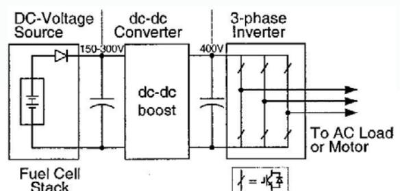
Figure 4: Traditional two-stage power conversion for fuel-cell applications
