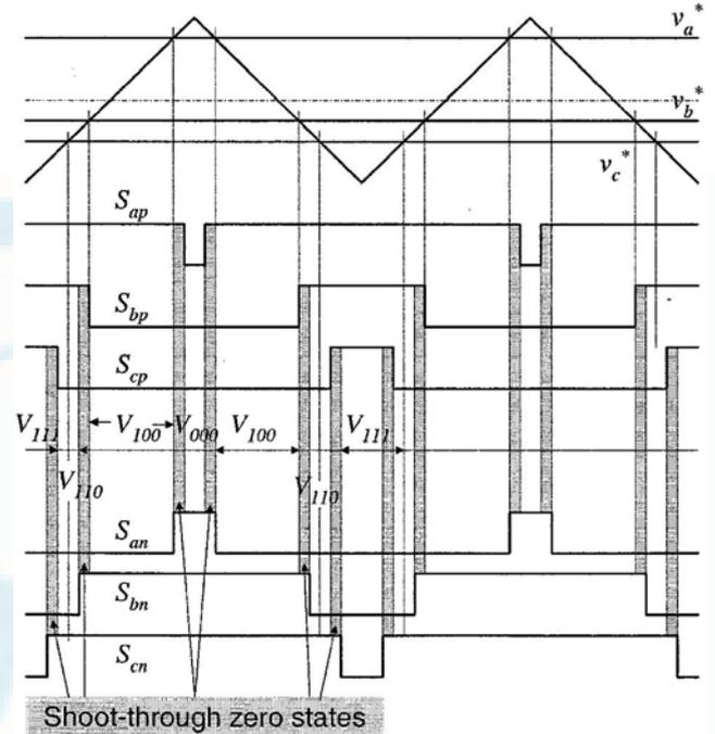
**Figure 10:** Modified carrier-based PWM control with shoot-through zero states that are evenly distributed among the three phase legs, while the equivalent active vectors are unchanged
