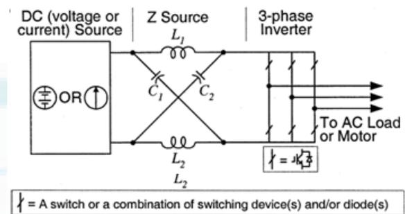
Figure 2: Z-source converter structure using the anti parallel combination of switching device and diode
