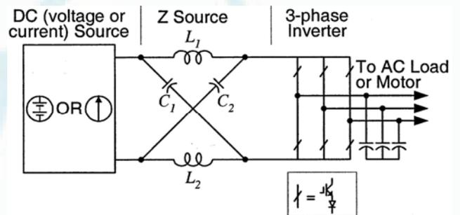
Figure 3: Z-source converter structure using the series combination of switching device and diode
