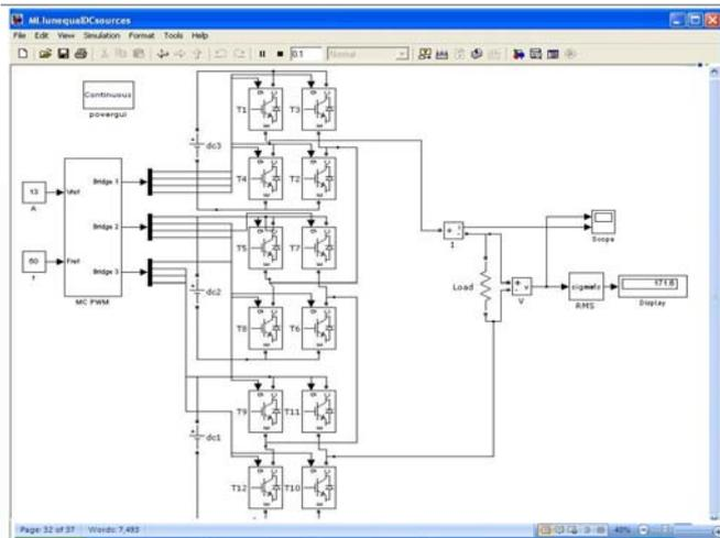
Figure 12: simulink diagram of the proposed system
