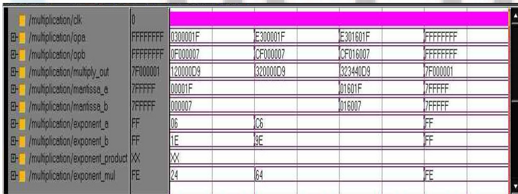
Figure 5: Simulation Waveform of Multiplication Code
