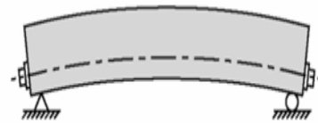
b. Post-tensioned concrete before loading
