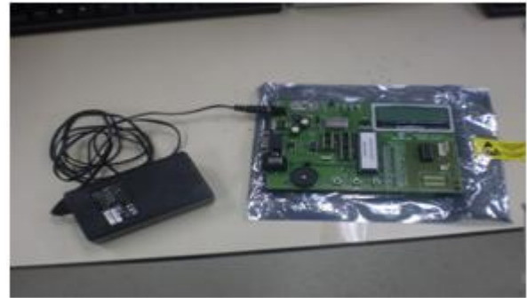
Figure 10: Connection of adaptor to J2 of board
