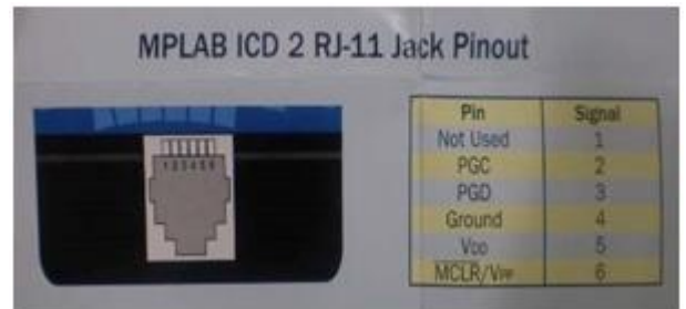
Figure 5: MPLAB ICD 2 RJ-11 Pin out (The MPLAB ICD 2 is connected to the PICDEM 2 Plus board using RJ-11)
