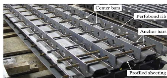
Figure 2: Photograph of profiled sheeting with perfbond ribs
