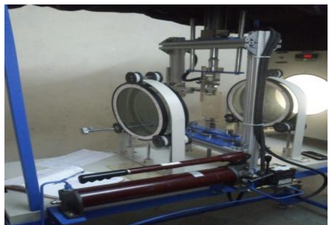
Figure 3: circular polariscope experimental setup
