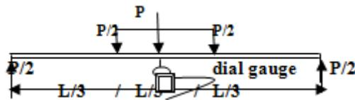
Figure 3a: A schematic beam testing setup
