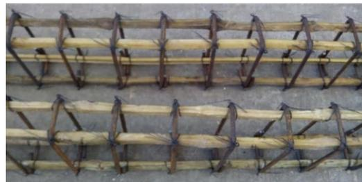
**Figure 1:** Treated bamboo reinforcement
