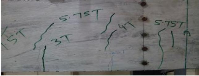
**Figure 4:** Nature of cracks formed
