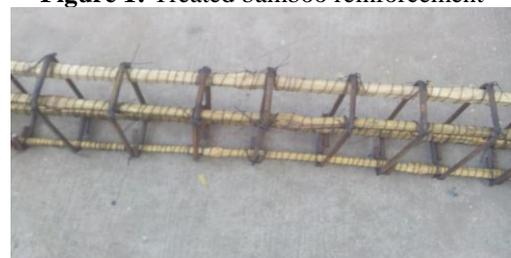
**Figure 2:** Treated bamboo reinforcement wrapped with binding wire
