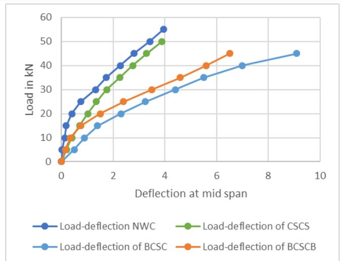
**Figure 5:** Typical load Vs Deflection graph for NWC, CSCB, BCSC, and BCSCB
