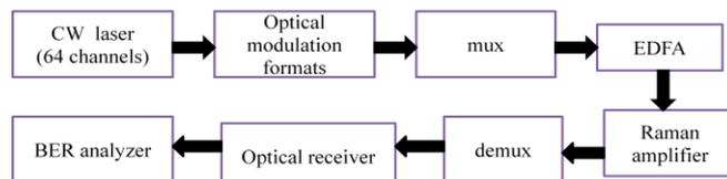
Figure 5: Hybrid configuration I
