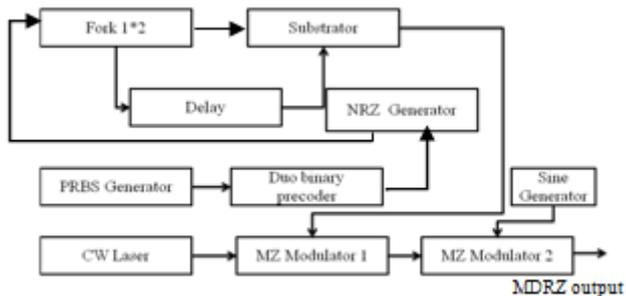
Figure 3: Modified Duo-Binary Return-To-Zero (MDRZ) format [8]
