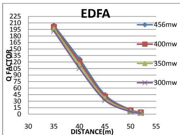
Figure 10: Distance vs Q factor of EDFA for various EDFA pump powers(mw)
