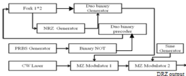
Figure 2: Duo-Binary Return-To-Zero (DRZ) format [8]
