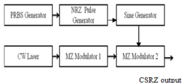
**Figure 1:** Carrier-Suppressed Return-To-Zero (CSRZ) format [8]
