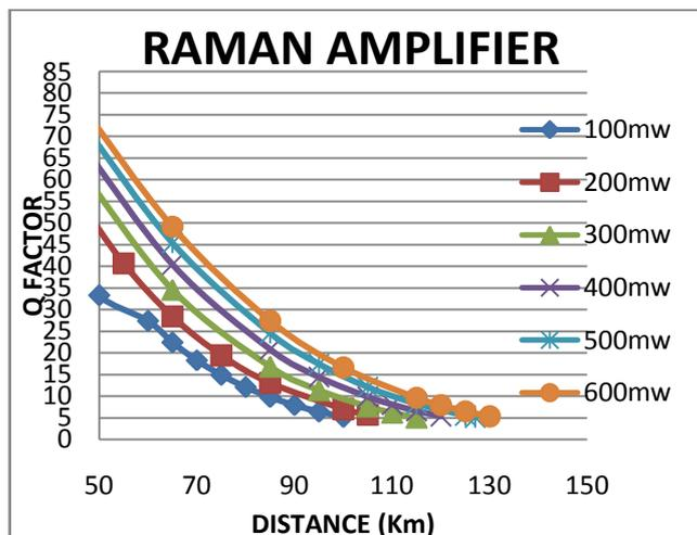
Figure 9: Distance vs Q factor of Raman amplifier for various Raman pump powers(mw)
