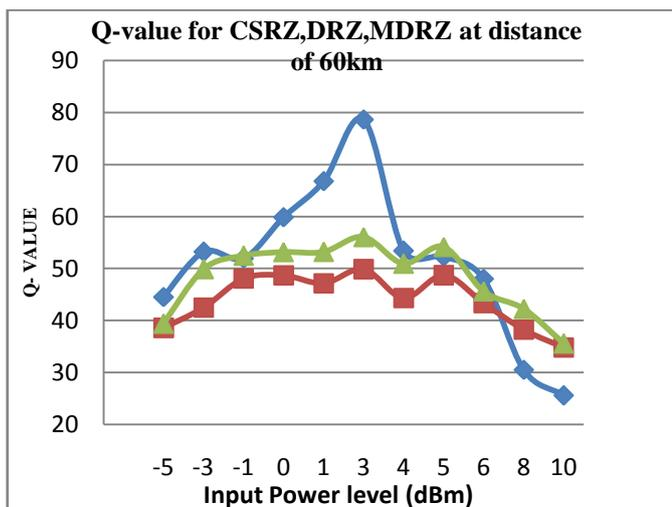
Figure 8: Variation of Q factor with respect to input power for various modulation formats for centre channel (Channel no. 32).
