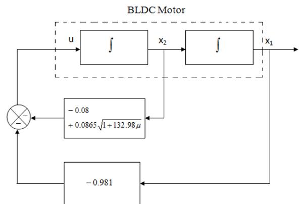
**Figure 2: Optimal Control of the BLDC Drive System**
