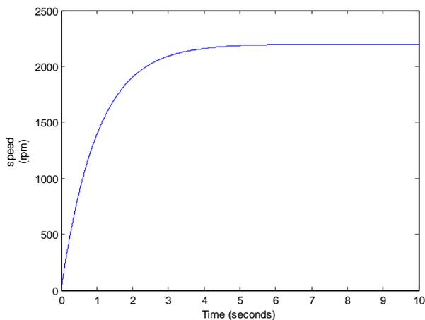
Figure 7: Tracking of BLDC motor at rated speed
