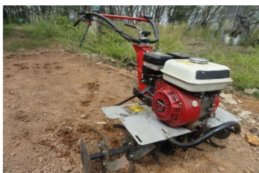
Figure 1: Photographic view of power weeder
