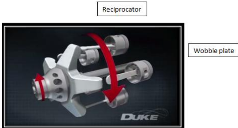
Figure 3: A reciprocator attached with wobble plate source dukeengines.com
