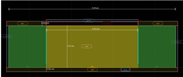
Figure 1: Structure of Planar MOSFET of channel length 22nm
