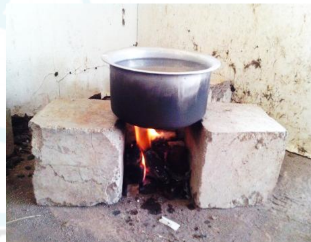
Figure 3: Three stone traditional cook stove
