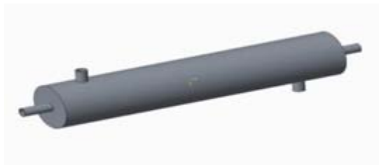
Figure 1: Single tube Parallel flow heat exchanger
