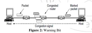
A special bit in the packet header is set by the router to warn the source when congestion is detected. The bit is copied and piggy---backed on the ACK and sent to the sender. The sender monitors the number of ACK packets it receives with the warning Bit set and adjusts its transmission rate accordingly.
