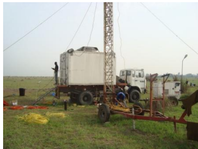
Figure 2: Exterior view of typical Seismic Recording Instrument Truck
