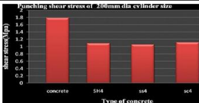
Figure 7: Punching Shear Stress of 200mm Diameter Cylinder at 12 days curing
