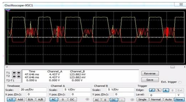
Figure 2: Multisim output signal of LC meter signal conditioning circuit to be sent to Atmega microcontroller
