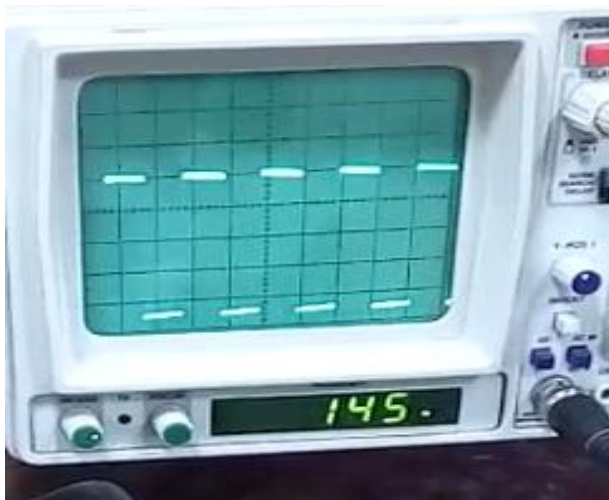
Figure 4 (b): Output frequency as observed in CRO in Capacitor mode.
