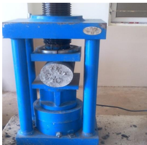
Figure 3: Split tensile Test on cylinders
