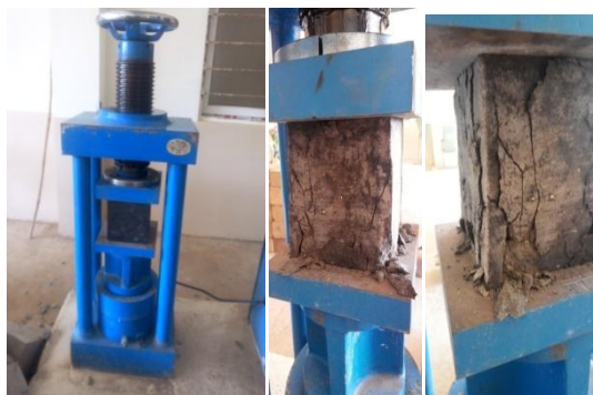
Figure 2: Compression Test on Cubes
