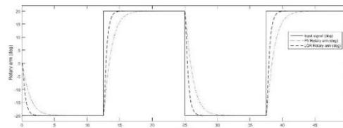
Figure 4.4.1: Response of Rotary arm
