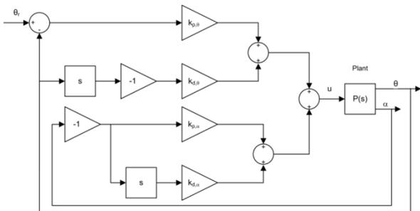
Figure 3.1.1: Block Diagram of PV Controller
