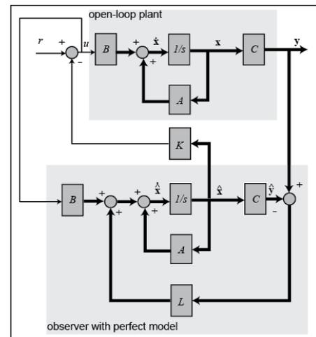
Figure 3.3.1: Block diagram of observer based control
