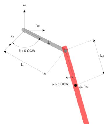
**Figure 2.1:** Free-body diagram of RIPS
