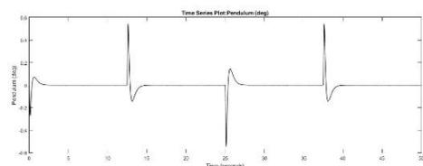
**Figure 4.2.3:** Response of pendulum
