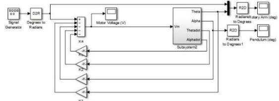
**Figure 4.2.1:** Simulink Model of an LQR Controller
