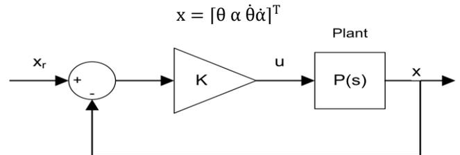
Figure 3.2.1: Block diagram of an LQR Controller
