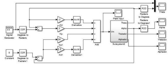
**Figure 4.1.1:** Simulink Model of PV Controller
