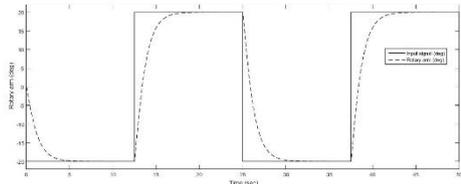
**Figure 4.1.2:** Response of arm for a PV Controller
