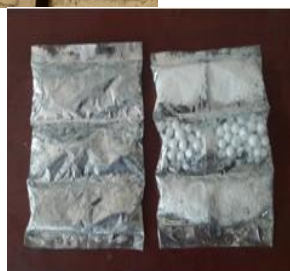
Figure 2: Macro encapsulation of PCM integrated into hollow block
