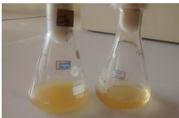
Figure 2: Inoculated sample and blank used for optical density.
