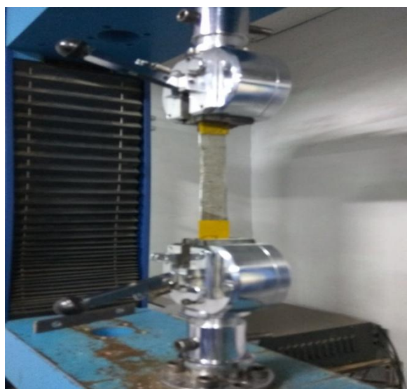
Figure 12: Specimen on UTM during tensile test
