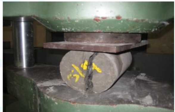
Figure 3: Split Tensile Strength on cylinder
