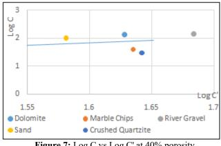
Figure 7: Log C vs Log C' at 40% porosity
