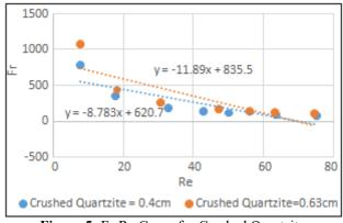
Figure 5: Fr-Re Curve for Crushed Quartzite
