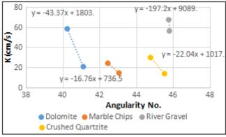
Figure 7: Angularity vs Hydraulic Conductivity
