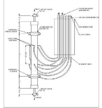
Figure 1: Details of permeameter set-up
