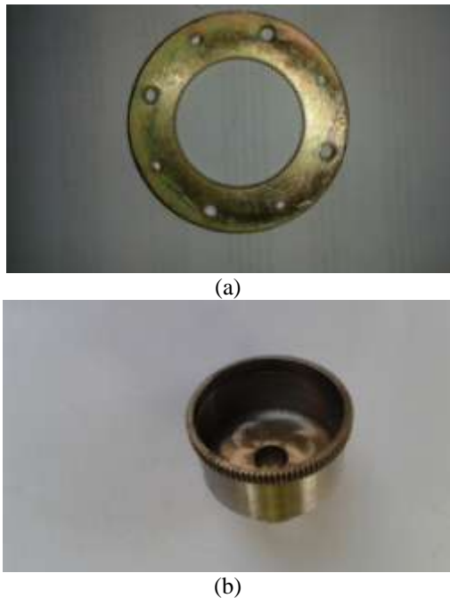
Figure 3.3: Photographs of Manufactured Harmonic Drive Components (a) Circular Spline (b) Flexspline
