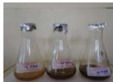
Figure 5: Samples after hot percolation method incubated for 3 hours at varying extract volume 0.5ml, 2.5 ml, 4.5ml
