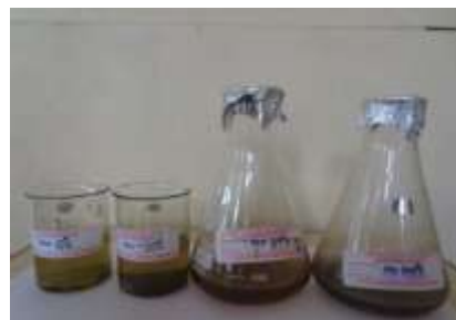
Figure 4: Samples after hot percolation treatment incubated for 3 hours at 4°C, 20°C, 37°C and 90°C
