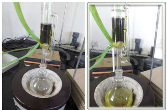
Figure 2: Soxhlet extraction of biofuel from oscillatoria
