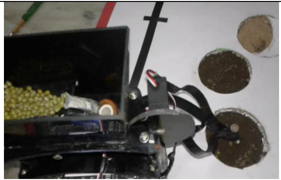
Figure 5.6: Robot making a hole and putting the seed in the field
