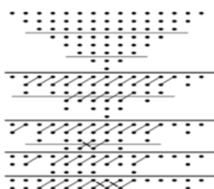
Figure 2: Example of Wallace tree reduction
