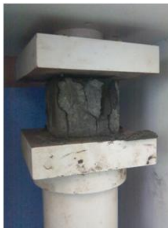
Figure 2: Testing of cubes in CTM
