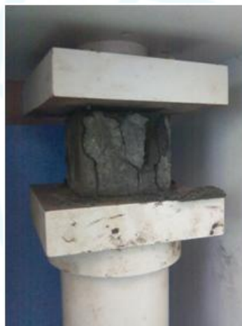
Figure 2: Testing of cubes in CTM
