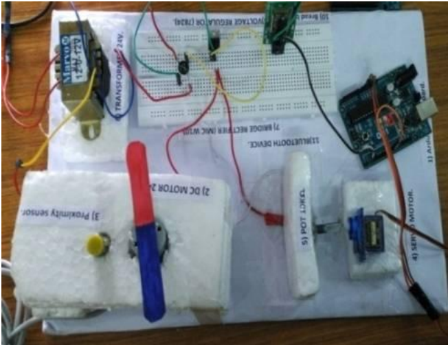
Figure 15: Hardware setup for Speed Control of DC Motor
