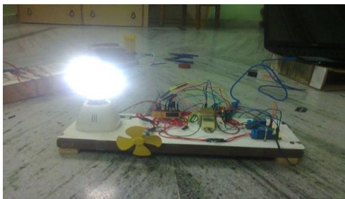
Figure 20: Load 2 (i.e. bulb) is in on position and load 1 (i.e. fan) is in off position
