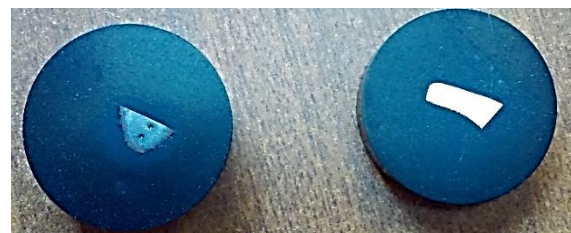
Figure 2: Mounted specimens (gear and piston)
